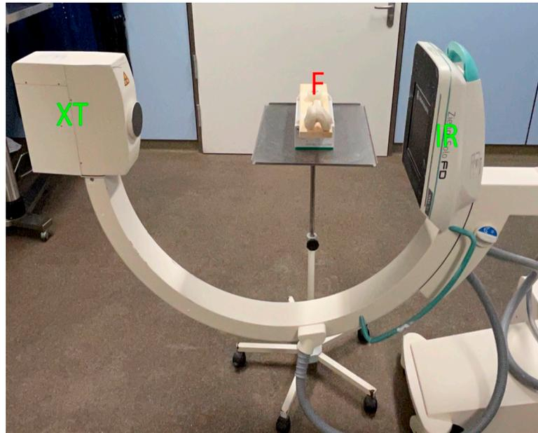
**Figure 1.** Femur positioning for the LM25 view of a right knee print. Contralateral positioning of the fluoroscopy. XT = X-ray tube, IR = image receptor, F = Femur.
