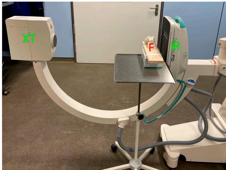
**Figure 2.** Positioning of the femur for the ML5 view of a right knee print. Ipsilateral positioning of fluoroscopy. XT = X-ray tube, IR = image receptor, F = Femur.
