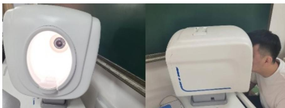
**Figure 7.** The device used for acquiring tongue images.
