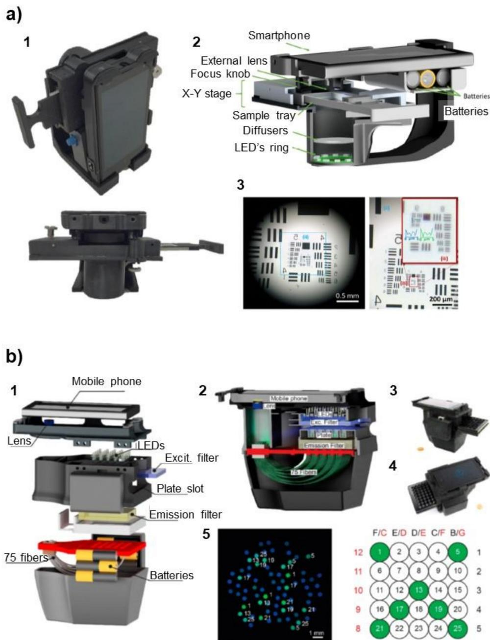
Figure 5. (a) Design of the smartphone microscope reported by Rivenson et al. 2018 (adapted with permission from [63];
