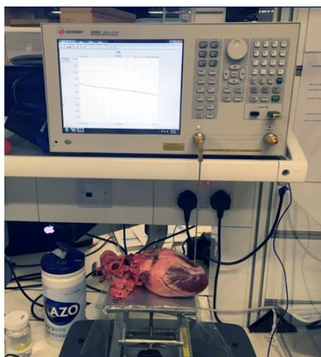
**Figure 1.** Measurement setup showing VNA2 directly connected to the slim form probe. The sample is brought in contact with the probe by lifting the table while making sure we do not apply excessive probe-sample pressure. The exclusion of the cable from the setup eliminates one source of measurement uncertainty.
