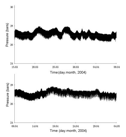
Figure 5. Pressure dynamics of water-steam mixture in well no. 30 in 2004. X-axis, day/month, Y-axis, pressure (bars).
