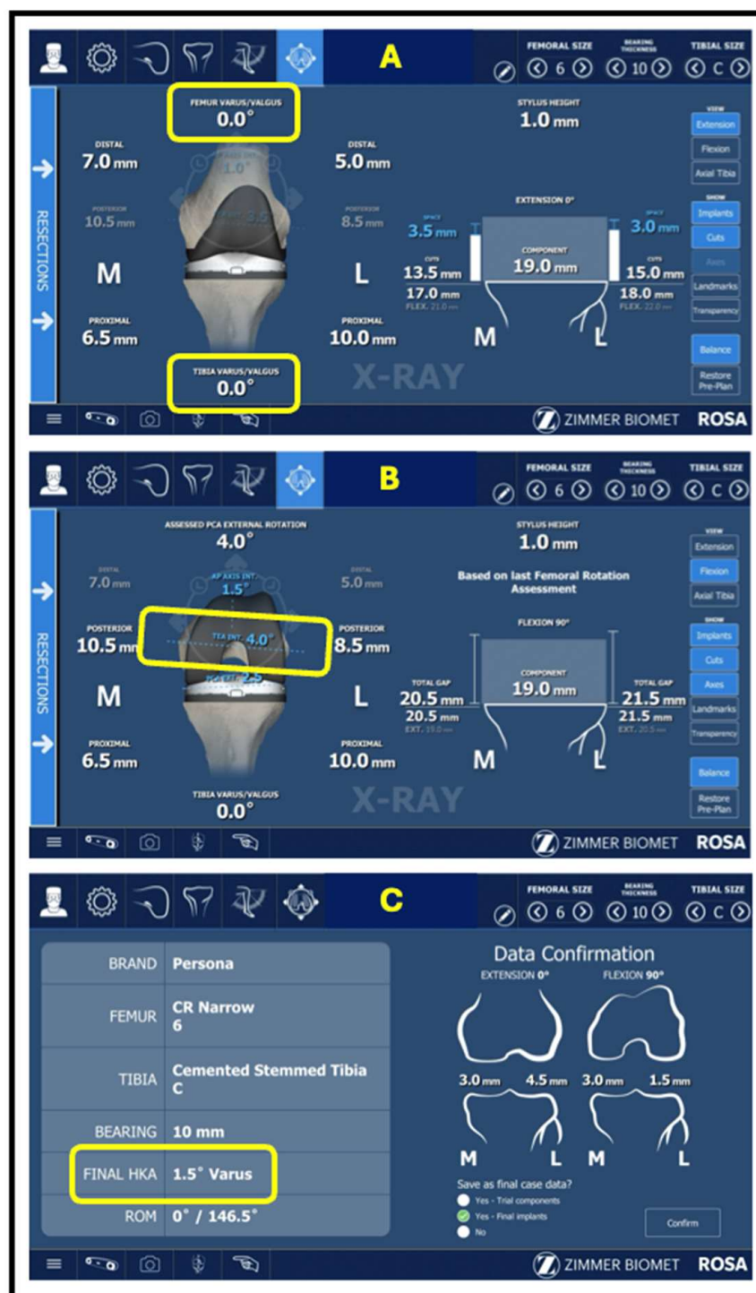
Figure 2. Example of patient data presented by ROSA Knee software intra-operatively. (A): Varus/valgus position of the femoral and tibial components highlighted. These values are used to calculate the LDFA and MPTA. (B): Femoral component external rotation visualized on this planning page intra-operatively. (C): Final HKA obtained is shown here and is used for comparison against the measured post-op HKA and aHKA.
