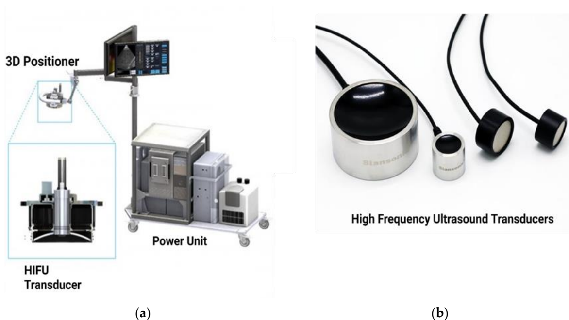
Figure 2. (a) FUS equipment. (b) HIFU transducers of varying sizes.
