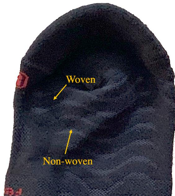
**Figure 1.** Woven and non-woven 3D waves (2 mm separation).
