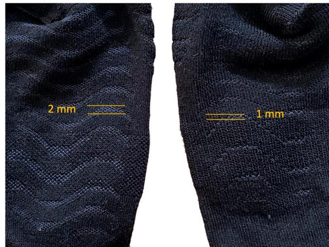
**Figure 3.** Type of wave separation: 2 mm for the socks on type 1 or AWC 2.2 (left) and 3 mm for type 2 or AWC 3 (right).
