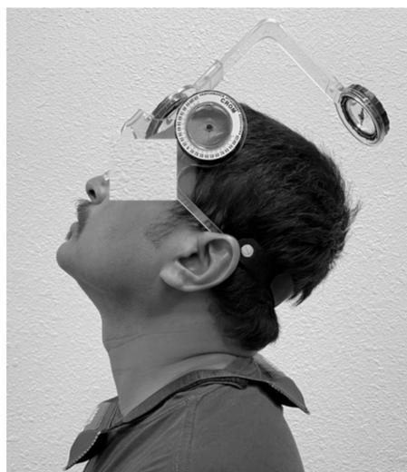
**Figure 1.** Cervical joint position sense testing using a CROM device.
