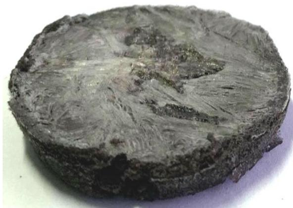
**Figure 1.** A GO/CS sponge after the freeze-drying process.
