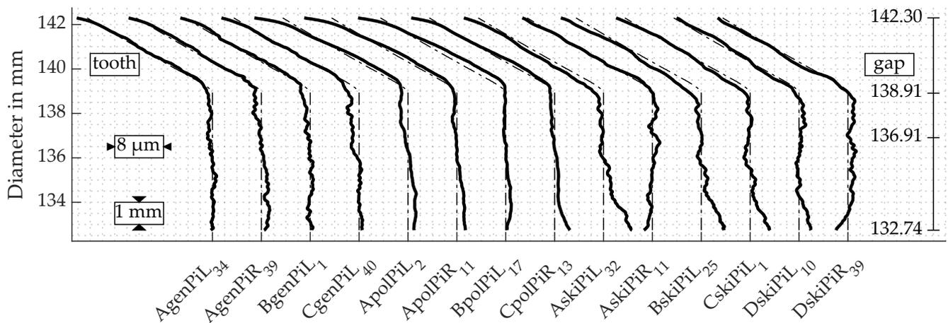
Figure 15. Profile lines of chosen teeth of all tested pinions.
