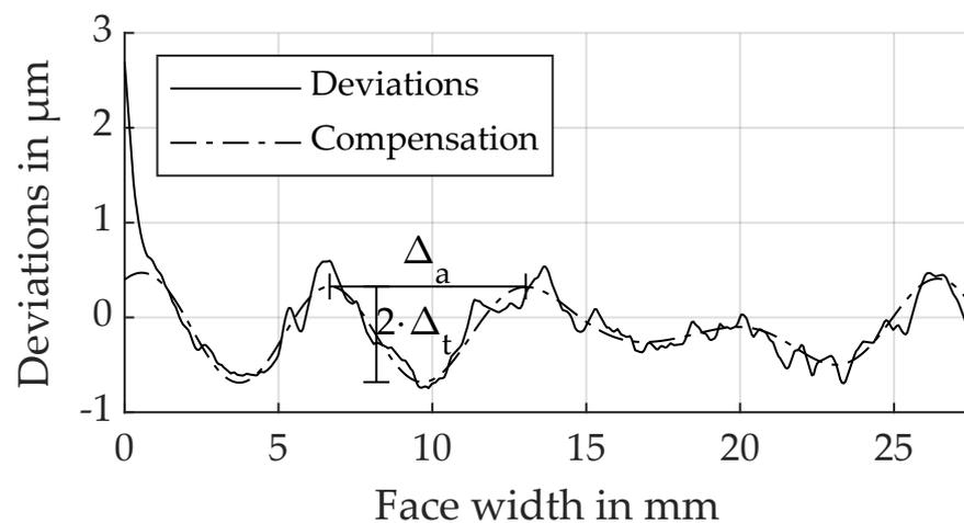
**Figure 4.** Distance and depth analysis of the largest regular deviations using a wavy compensation curve (the diagram shows DskiPiLZ at tooth nr. 10).
