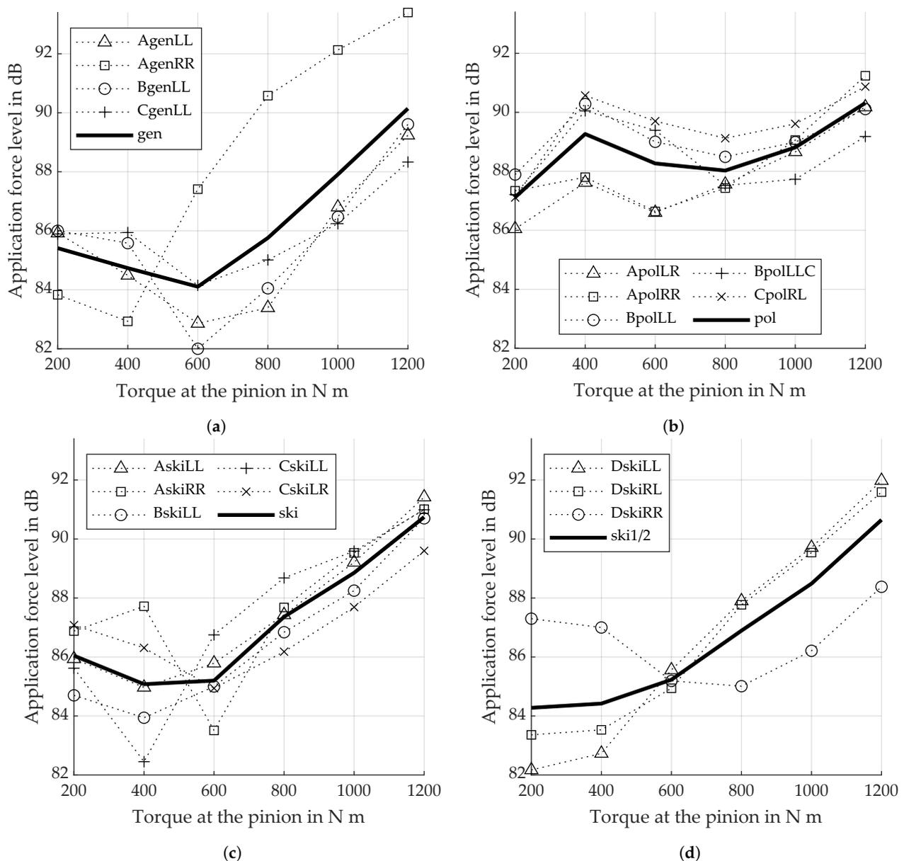
**Figure 19.** Application force level from torsional acceleration measurement of the different manufacturing processes. (a) Continuous generating grinding. (b) Polish grinding. (c) Gear skiving. (d) Gear skiving with half axial feed.
