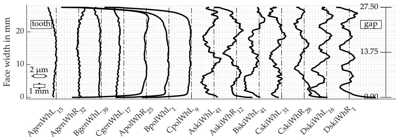
Figure 18. Lead lines of chosen teeth of all tested wheels.
