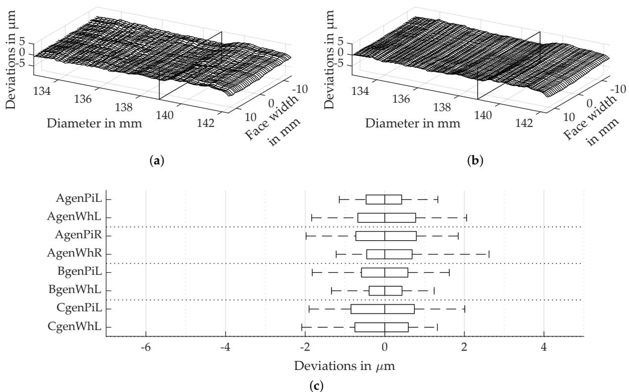
**Figure 10.** Deviations for continuous generating grinding. (a) Flank of gear AгенPiL at tooth nr. 34. (b) Median of all teeth of gear AгенPiL. (c) Box plot of the deviations in the gear pairs.
