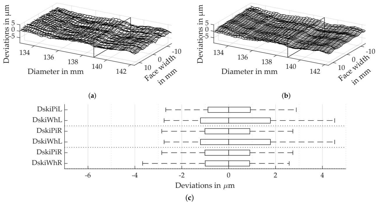
**Figure 13.** Deviations for gear skiving with half of the axial feed. (a) Flank of gear DskiPiL at tooth nr. 10. (b) Median of all teeth of gear DskiPiL. (c) Box plot of the deviations in the gear pairs.
