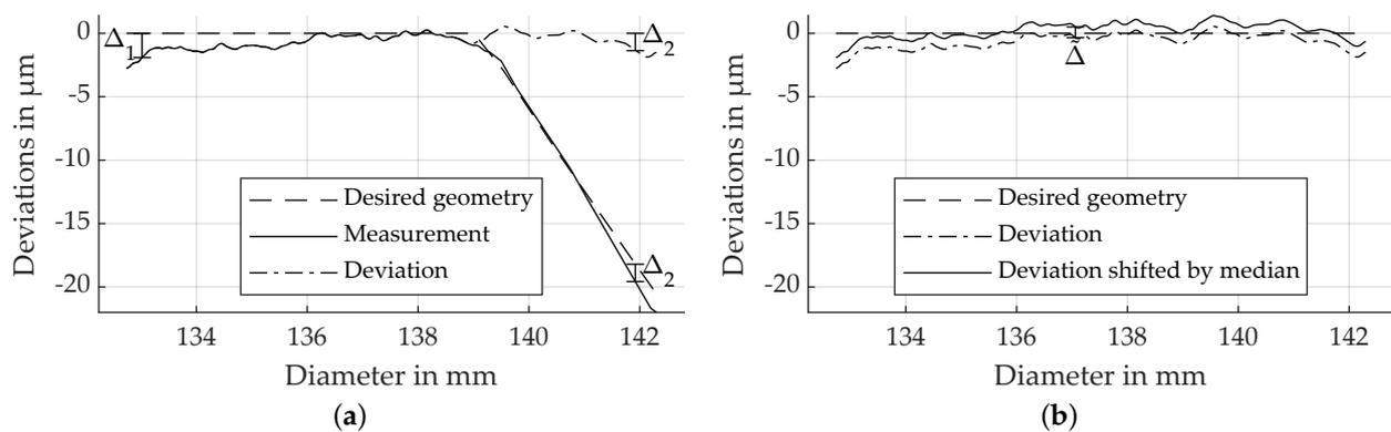
**Figure 3.** Procedure to obtain the deviations used in this study out of the measured flank and the desired geometry. (a) The desired geometry is deduced from the measured profile line in order to obtain the resulting deviations (resulting deviations at two diameters see  $\Delta_1$  and  $\Delta_2$ ). (b) In order to compare the results with the other flanks, the resulting deviations are shifted by the median of the deviations in a single flank  $\bar{\Delta}$ .
