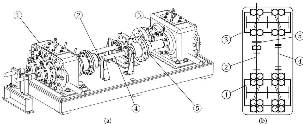
**Figure 6.** FZG dynamic test rig: 1-test gearbox, 2-pinion shaft, 3-drive gearbox, 4-wheel shaft, 5-loading clutch. (a) CAD view. (b) Principle sketch.
