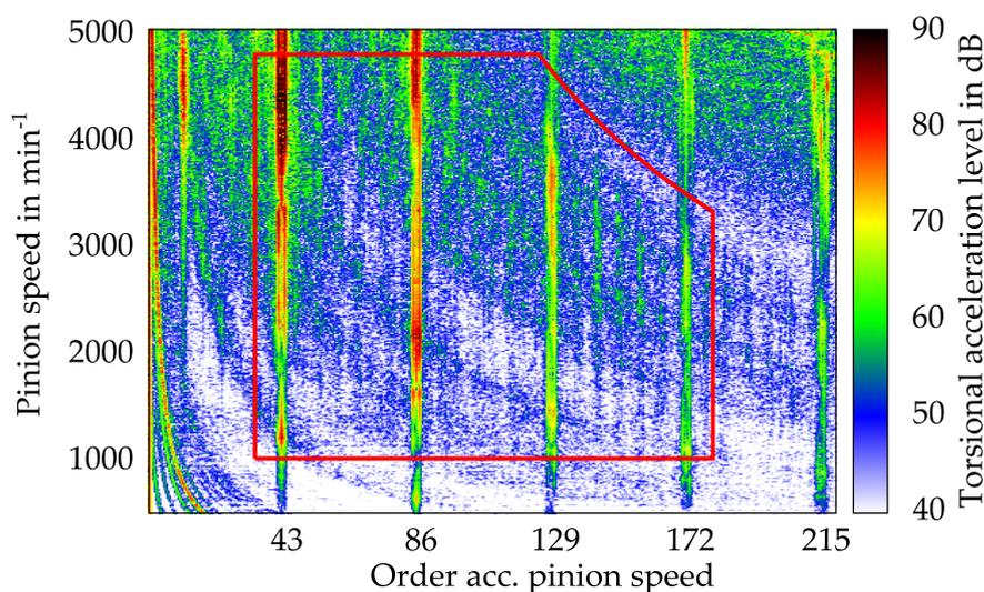
**Figure 8.** Exemplary Campbell-diagram with leveled amplitudes, that shows the torsional acceleration measurement of polish ground gears at 800 N m. The relevant operating range for the application force level is marked with red lines.
