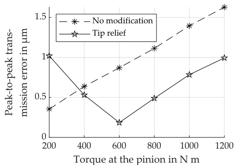
**Figure 2.** Peak-to-peak transmission error of the gear pair used in the experiment.
