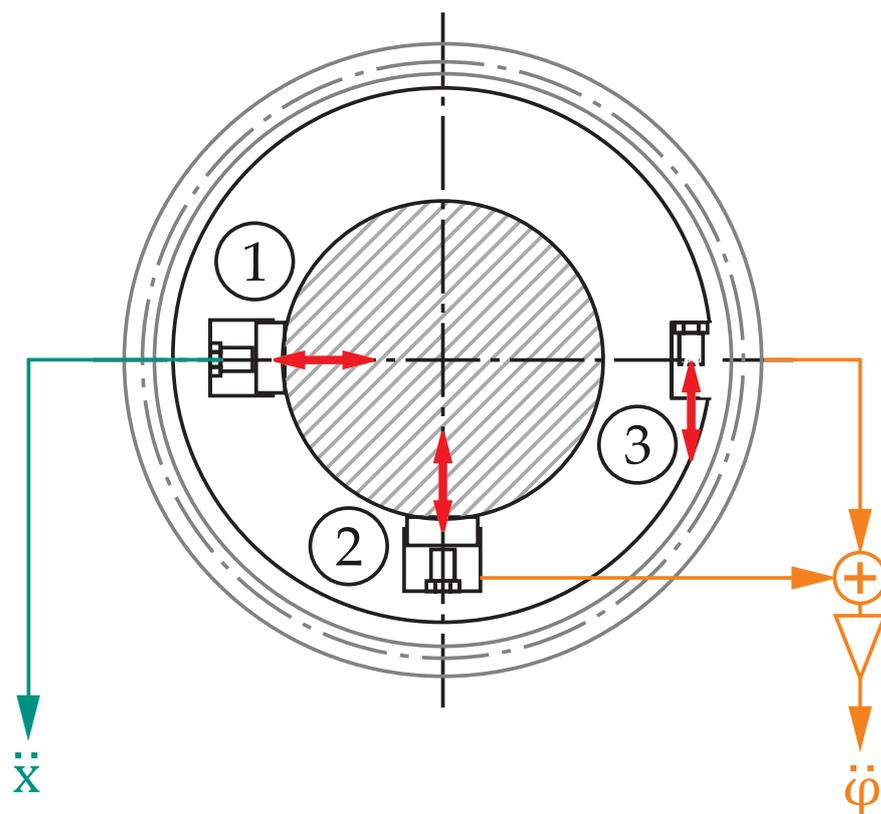
**Figure 7.** Measurement disc and sensor position for torsional acceleration measurement: 1–2-radial sensors, 3-tangential sensor according to [9].
