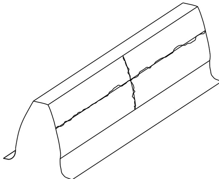
**Figure 14.** Location of the profile and lead line measurement at the gear flank.
