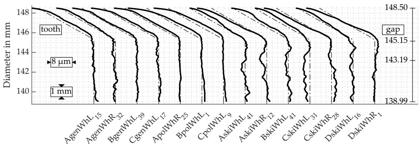
Figure 16. Profile lines of chosen teeth of all tested wheels.
