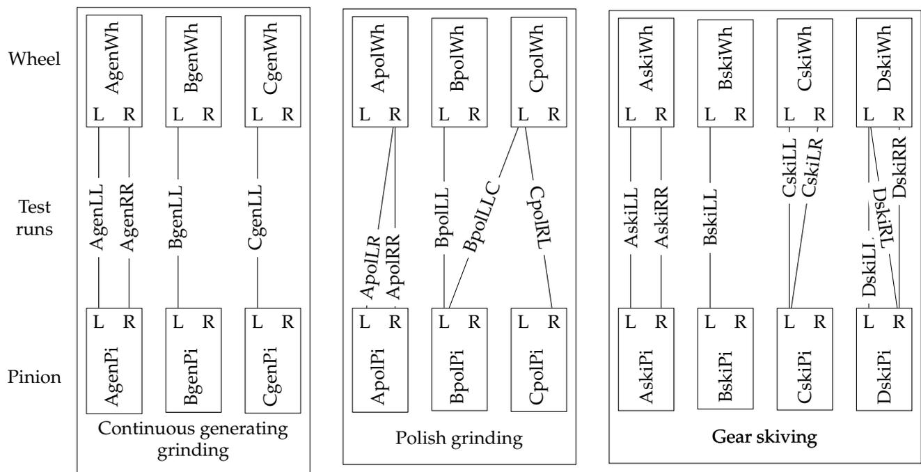
**Figure 9.** Overview of the active flanks of the gears in the test runs
