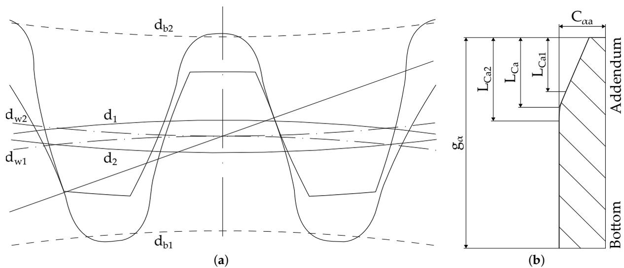
**Figure 1.** Gear pair used in the experiment. (a) Profile of the gear pair in transverse section. (b) Linear tip relief with parabolic transition.
