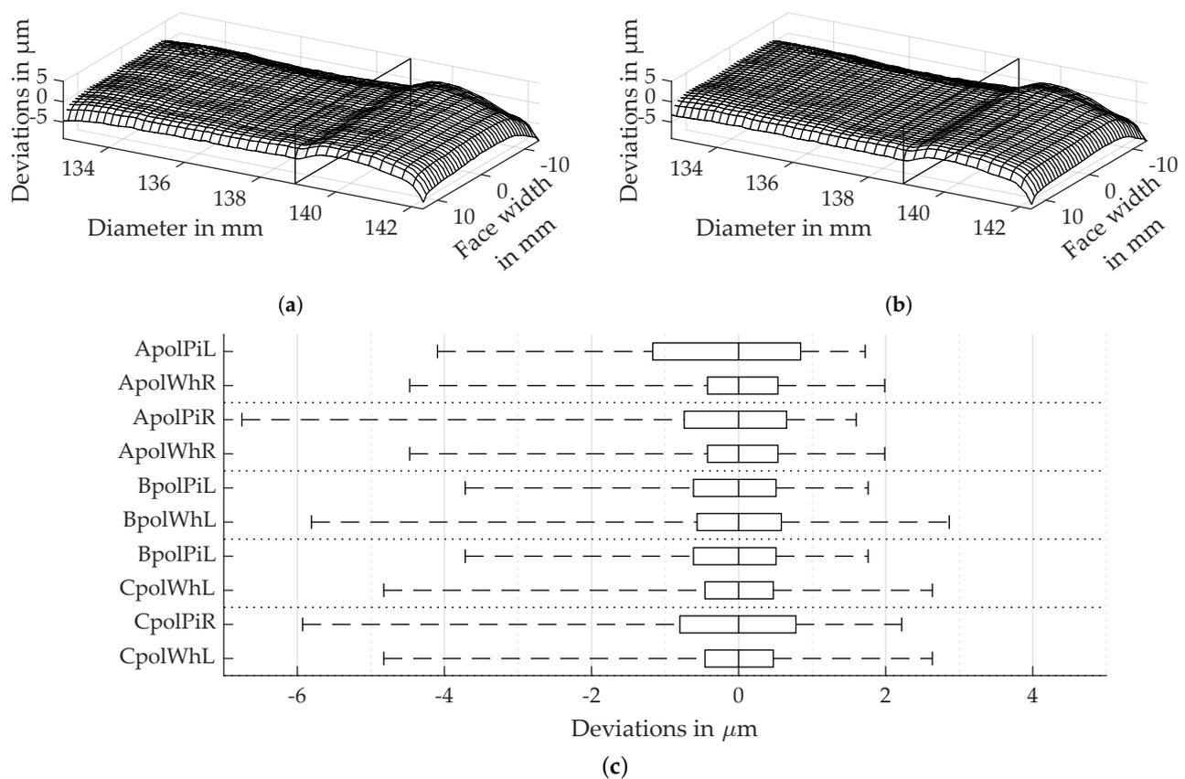
**Figure 11.** Deviations for polish grinding. (a) Flank of gear BpolPiL at tooth nr. 17. (b) Median of all teeth of gear BpolPiL. (c) Box plot of the deviations in the gear pairs.
