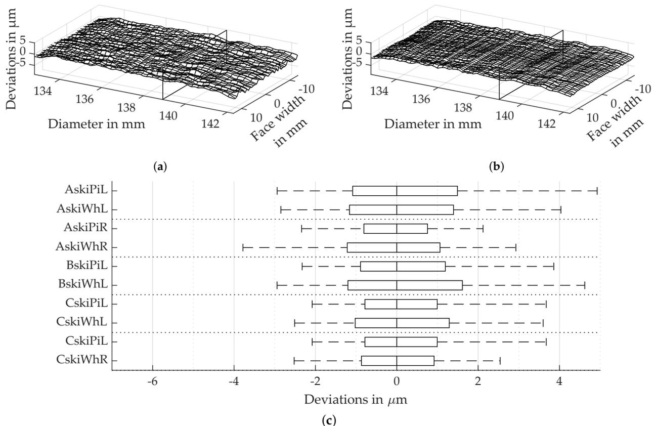
**Figure 12.** Deviations for gear skiving. (a) Flank of gear AskiPiR at tooth nr. 11. (b) Median of all teeth of gear AskiPiR. (c) Box plot of the deviations in the gear pairs.
