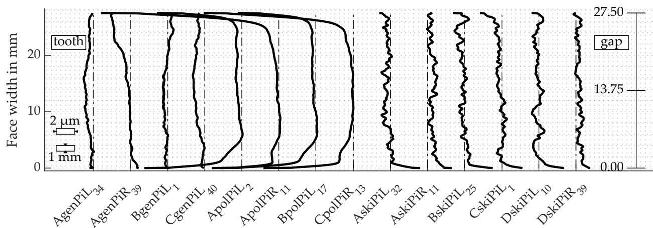
Figure 17. Lead lines of chosen teeth of all tested pinions.
