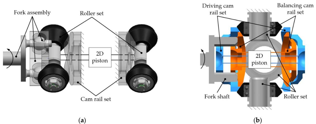
**Figure 1.** Schematic diagram of the 2D transmission mechanism: (a) the overall architecture of the 2D transmission mechanism; (b) the 2D transmission mechanism with inertial force balanced.
