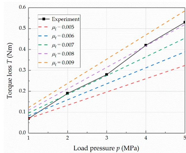
**Figure 18.** Analytical and experimental torque losses with respect to the load pressure at the rotational speed of 10,000 rpm.
