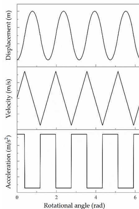
**Figure 5.** The motion law of the cam rail set.
