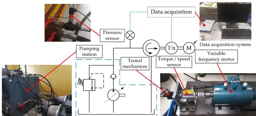
Figure 17. Schematic diagram of the experiment rig.
