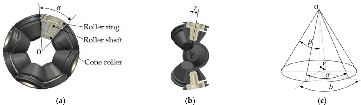
**Figure 3.** Structure principle of the stacked roller set: (a) front view of the stacked roller set; (b) side view of the stacked roller set; (c) projection of the cone roller.
