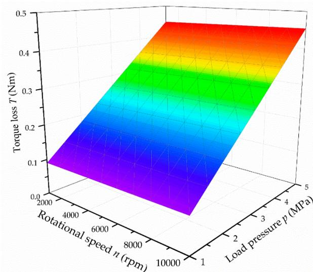
**Figure 16.** Theoretical torque characteristics.
