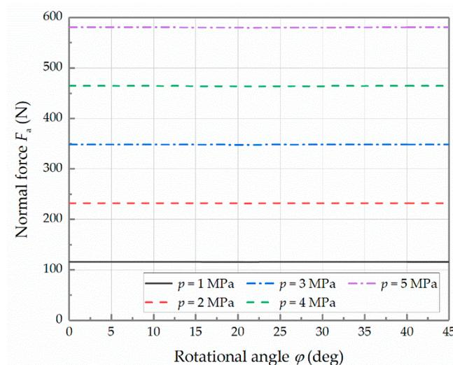
**Figure 12.** Curves of the normal force  $F_a$  at different pressures.
