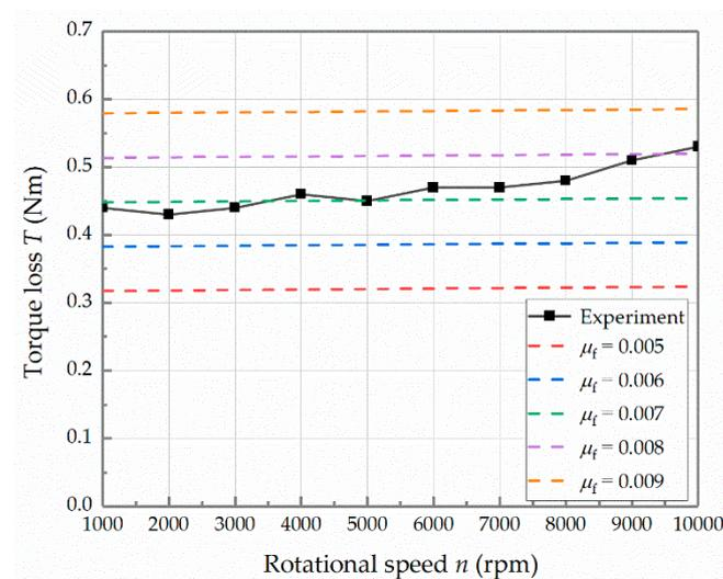
**Figure 19.** Analytical and experimental torque losses with respect to the rotational speed at the load pressure of 5 MPa.
