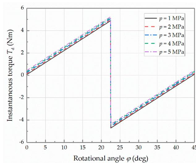
**Figure 13.** Curves of the instantaneous torque at different pressures.
