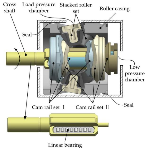
**Figure 2.** Structure of the high-speed transmission mechanism with a stacked roller set.
