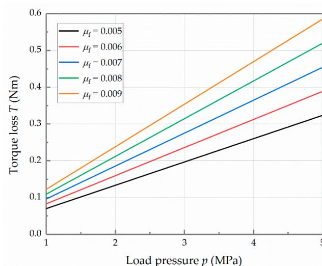
**Figure 14.** Curves of the torque loss with respect to the load pressure at different friction coefficients.
