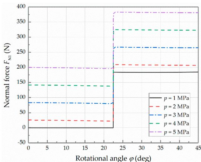
Figure 10. Curves of the normal force  $F_{N1}$  at different pressures.
