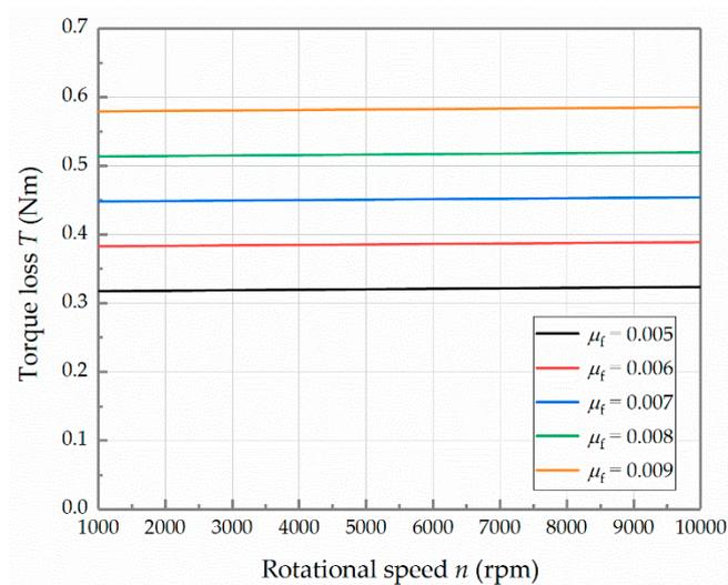
**Figure 15.** Curves of the torque loss with respect to the rotational speed at different friction coefficients.
