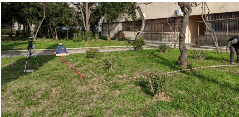
**Figure 9.** The experimental arrangement deployment being necessary for testing the path-following accuracy of the proposed robotic vehicle on both smooth and comparatively rough terrains.
