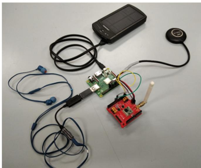
**Figure 6.** An indicative arrangement allowing for voice command functionality and GPS positioning using a raspberry pi 3 model A+, a LoRa Dragino radio module, and the ASUS AI noise-canceling stick plus a headset. This system variant is tailored for accompanying the operator (i.e., the farmer).
