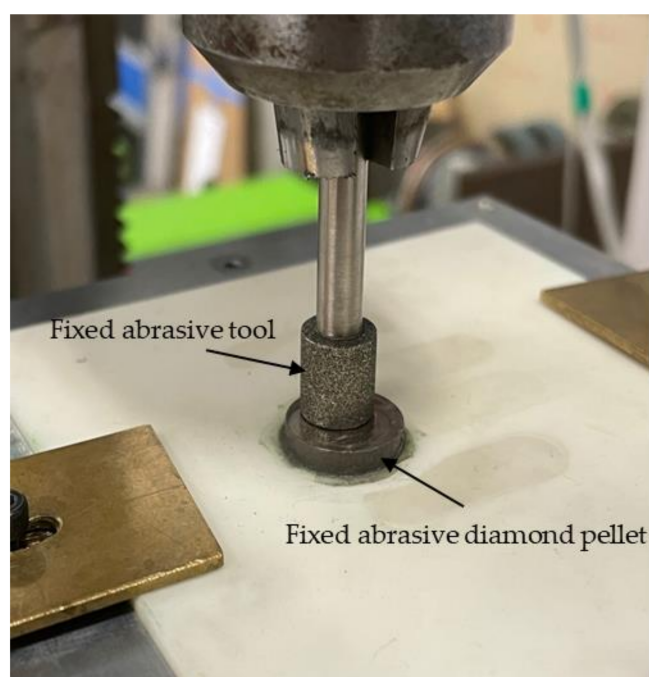
Figure 7. Pretreatment of fixed abrasive tool.
