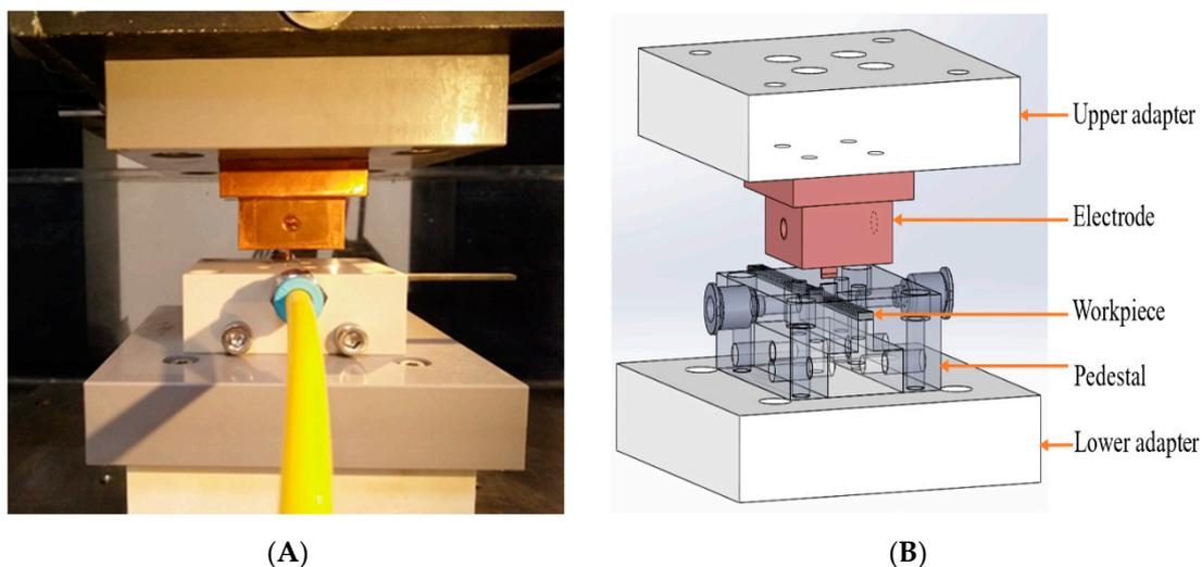
**Figure 2.** The structure of the electrode module: (A) actual device used during experimentation and (B) 3D design of the electrode module.
