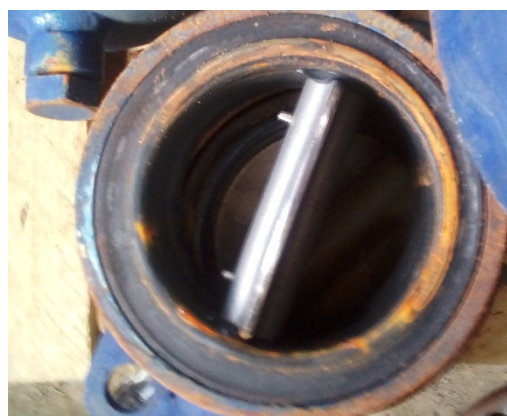
Figure 15. A heat supply system equipment (a valve) if geothermal water is treated with an acoustic-magnetic device.
