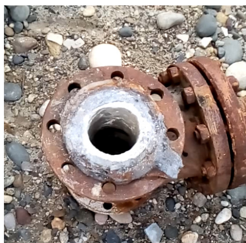
Figure 14. Deposits formation on a heat supply system equipment if geothermal water is not treated with an acoustic–magnetic device.
