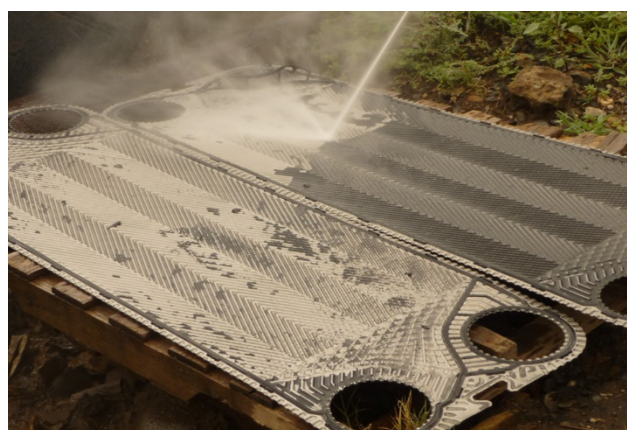
Figure 13. The cleaning process of heat exchanger plates (of a heat supply system with acoustic–magnetic devices).
