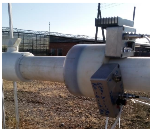
Figure 12. Acoustic–magnetic device installed on a pipe of heating main.
