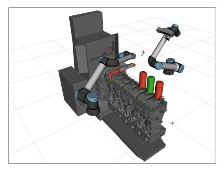
**Figure 7.** Simulation showing experiment E7. In this experiment, the robot to the left, *r*2, has stopped responding for an unknown reason. However, it is still attached to the smart tool (orange), which is needed to complete assembly. Additionally, *r*2 is physically blocking the space around the bolts.
