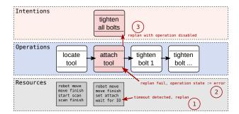
Figure 6. Propagating errors in the hierarchy.
