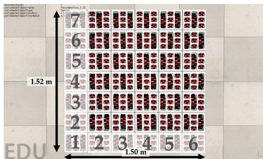
Figure 6. A top view screenshot of the proposed E-pattern omniwheeled cellular conveyor (EOCC) platform in V-REP environment.
