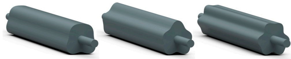
Figure 4. Rotors with harmonic roundness component pairs. On the left: components 3 and 4, in the middle: components 3 and 5, on the right: components 3 and 6.
