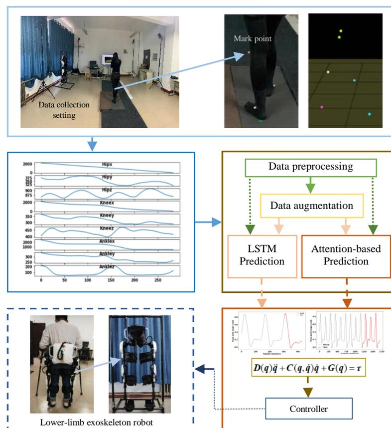
Figure 1. Gait trajectory prediction for lower-limb exoskeleton rehabilitation.
