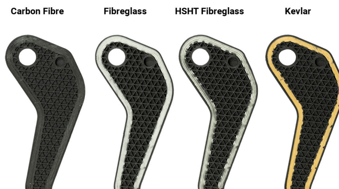
Figure 1. Presentation of cross-sections of composite prints using various reinforcing materials, from the left: carbon fiber, glass fiber, high-strength high-temperature glass fiber and Kevlar [16].
