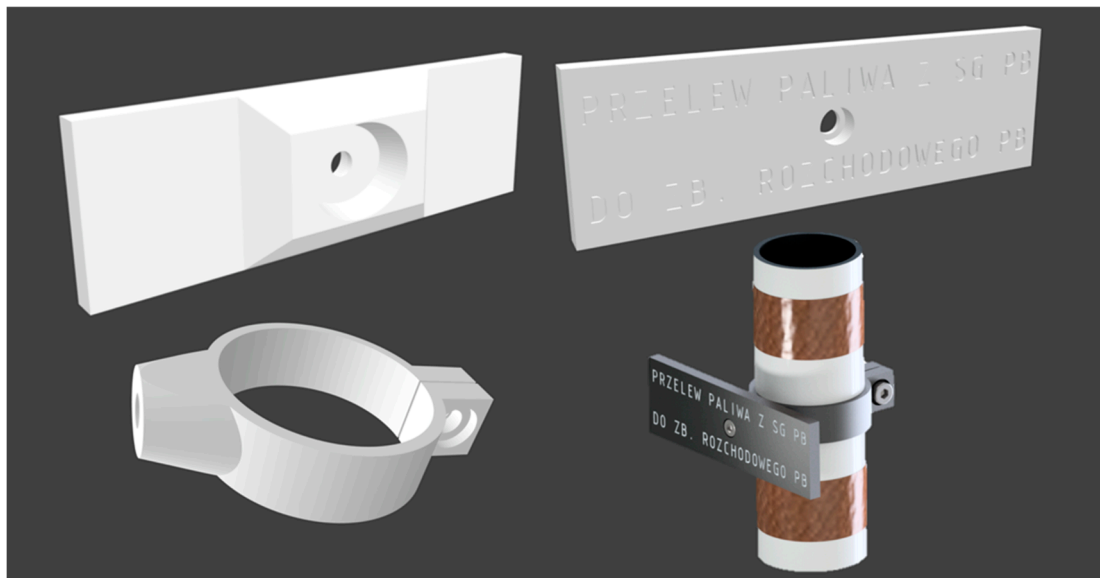
Figure 16. Models of the designed name plate and the mounting. From the top: name plates, view from the back and front, the mounting and the assembly of all components.
