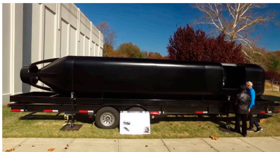
Figure 12. Submarine hull made incremental techniques for the US Navy [41].
