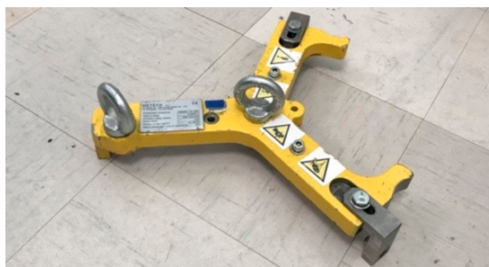
Figure 13. Mounting previously used by Wärtsilä personnel [42].
