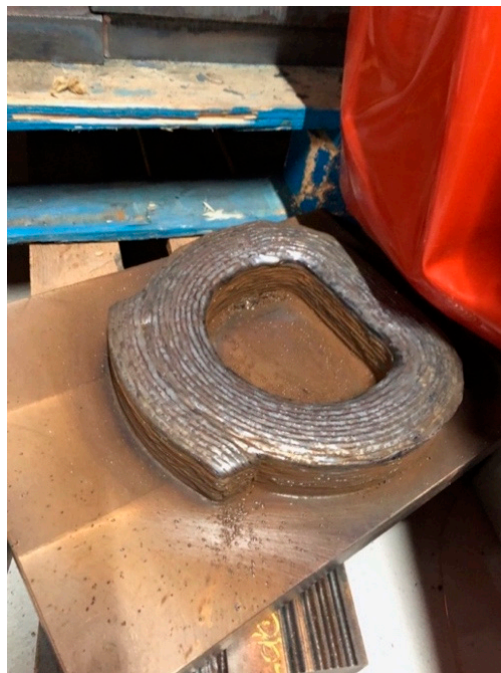
Figure 10. Crane hook during the 3D printing process.
