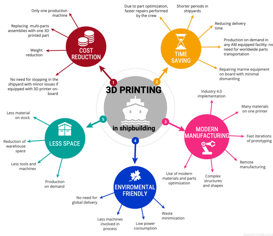
Figure 20. Graphic representation of the benefits of using 3D printing in shipbuilding.
