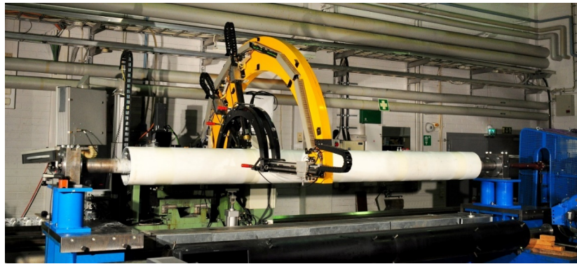
Figure 6. The measurement setup to capture dynamic responses was built on a commercial roll grinding machine [18].
