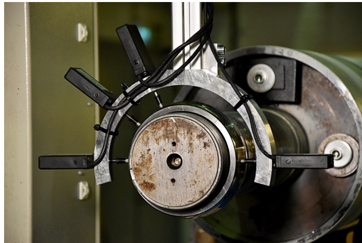
Figure 4. The bearing inner ring roundness profile was measured while installed on the rotor shaft [24].
