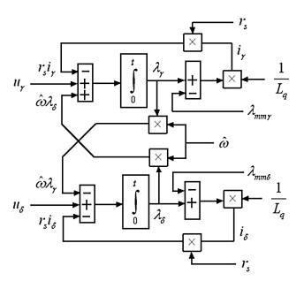
**Figure 6.** The PMSM model in  $\gamma\delta$  reference frame that is used as basis to form the sliding mode observer (SMO) for speed and position estimation.
