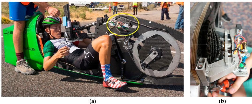
**Figure 4.** First prototype of the moving cassette: (a) the HPV Taurus at the WHPSC 2017 with the first moving cassette shifter on the right side (photo courtesy of F. Corda); and (b) close-up view (photo courtesy of J. Nogami).
