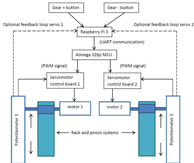
**Figure 7.** Layout and logic of the electronic control.
