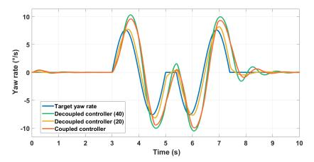
Figure 21. Different controllers for the yaw rate.
