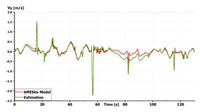
Figure 7. Validation of the vehicle model: lateral speed [10].
