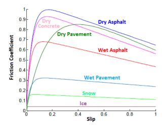
Figure 26. Friction coefficient for different surface types [33].
