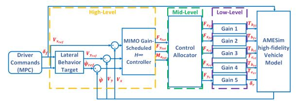
Figure 12. Vehicle motion multi-layered control architecture.
