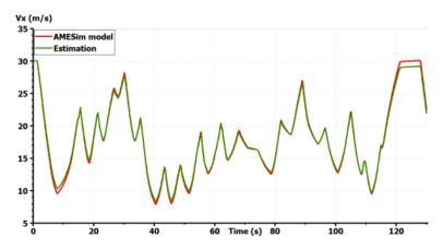
Figure 6. Validation of the vehicle model: longitudinal speed [10].
