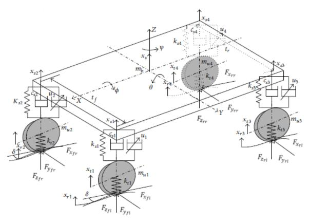
Figure 3. 1four-DoF vehicle dynamic model (adapted from [2]).
