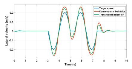
**Figure 23.** Lateral speed control using GS  $\mathcal{H}_{\infty}$ .
