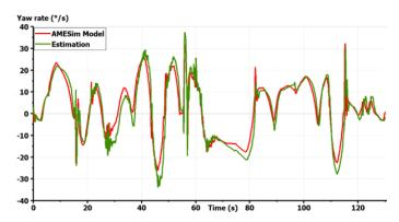
Figure 11. Validation of the vehicle model: yaw rate [10].
