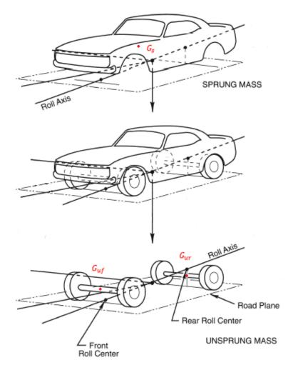
Figure 2. The sprung and unsprung masses decomposition.
