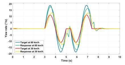
**Figure 22.** Various speed control using GS  $\mathcal{H}_{\infty}$ .
