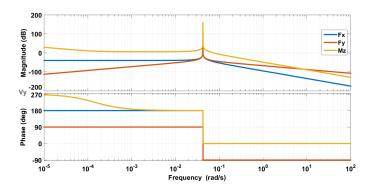
Figure 14. Bode diagrams for the lateral velocity [10].
