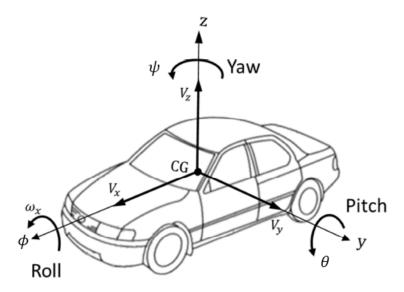
Figure 1. Vehicle Axis System ISO 8855-2011.
