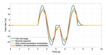
Figure 20. Robustness of the controller against parameters uncertainties.
