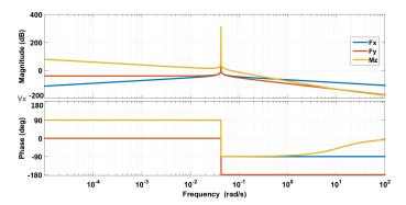
**Figure 13.** Bode diagrams for the longitudinal velocity [10].
