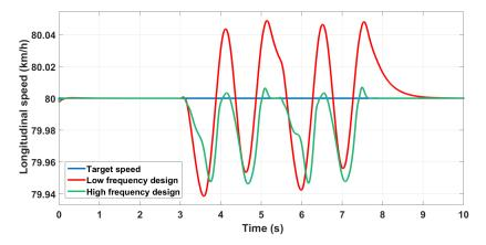
Figure 18. Longitudinal velocity control with different crossover frequencies.
