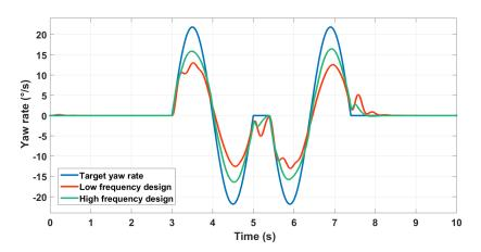
Figure 19. Yaw rate control with different crossover frequencies.
