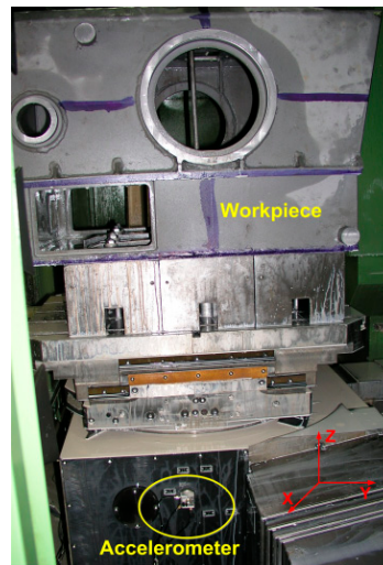
Figure 5. The sensor installation.
