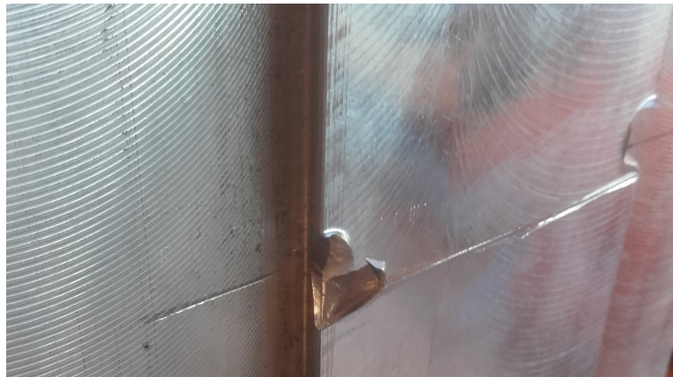
Figure 16. Picture of a damaged wedge on the pipe, the result of a failed mounting attempt that happened early on during the development of the system, where a poorly aligned pole-shoe was being forced onto the pipe at too high speed.
