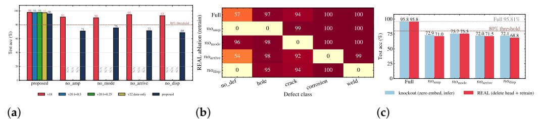
Figure 9. Three cross-cutting views of the ablation study on the 5000-sample test set. (a) Scheme-level: The proposed baseline (dark blue) at 95.05% together with its four knockout ablations, all collapsing below the 80% hard-requirement threshold (68.79–75.55%). (b) Per-class knockout heatmap: Diagonal collapses with off-diagonal side-effects on no-defect/hole ( ko_{amp} ) and no-defect/weld ( ko_{disp} ) reveal that the four physics heads are entangled at the representation level. (c) Real-ablation accuracy across the four segments (71.05/75.55/71.55/68.79% under the corrected val-best protocol), all below the 80% threshold line, demonstrating that the proposed architecture cannot maintain industrial-acceptance accuracy when any single physics head is removed.
