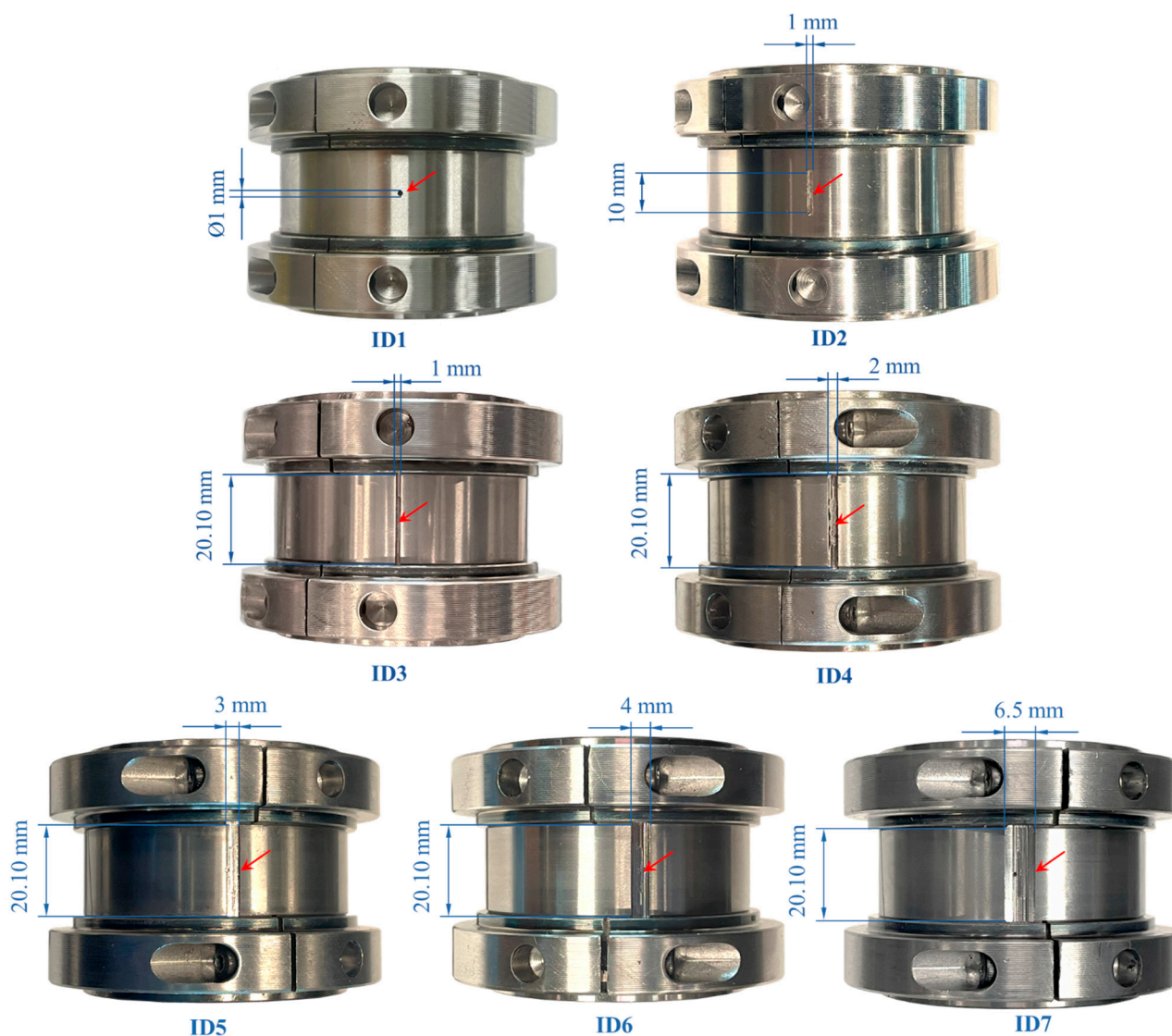
Figure 11. Inner-race defects (as marked by red arrows).
