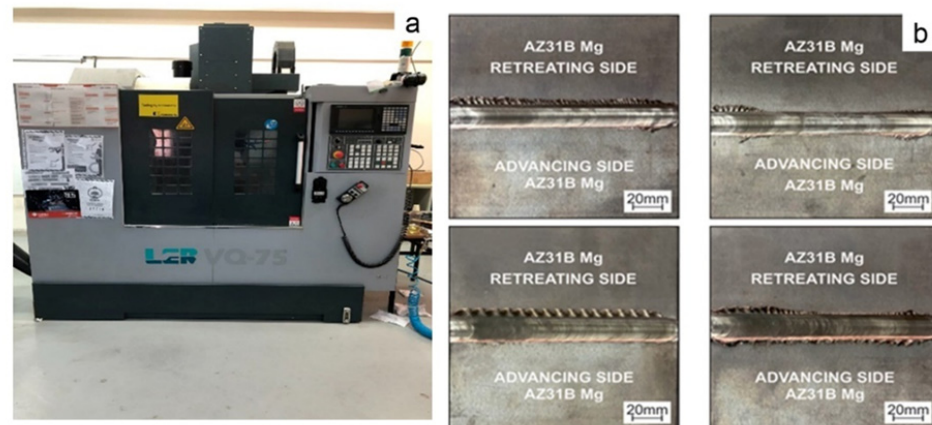
Figure 3. Experiment setup, illustration of typical weld bead surface appearance (a) universal milling machine (LER VQ75) used in FSW experiment, (b) weld surface under different process conditions [23].
