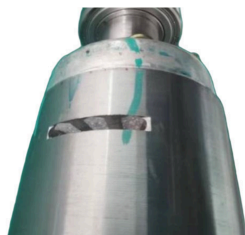
Figure 21. Broken rotor bar fault.
