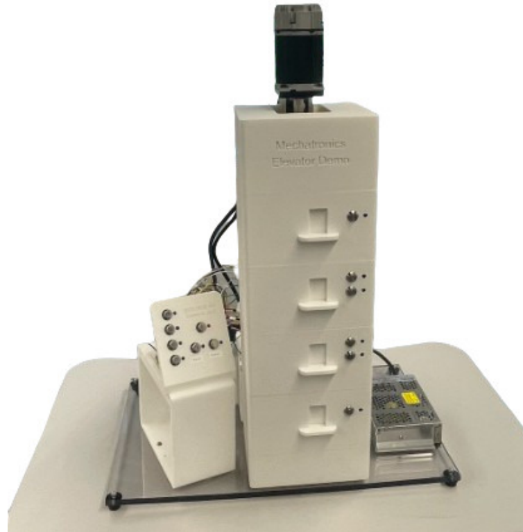
Figure 1. Completed elevator model with four floors and a panel (left) to represent the inside buttons.
