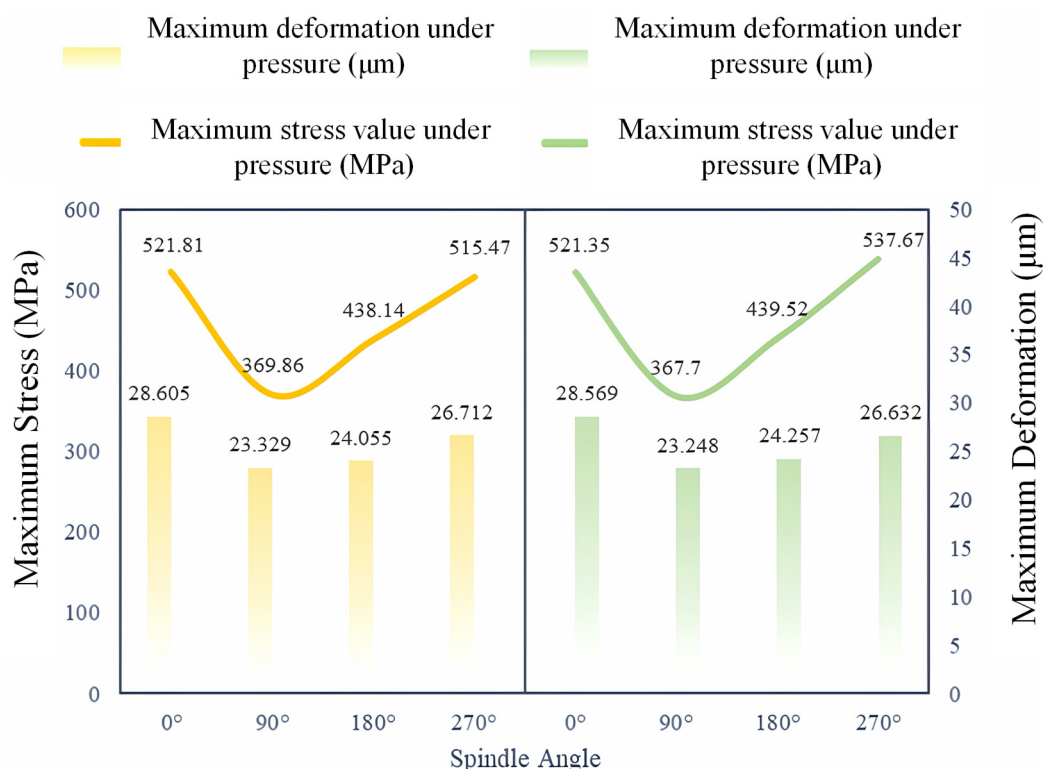
Figure A6. The variation trends of the maximum deformation and the maximum stress value at different spindle rotation angles under the action of temperature load and under the action of temperature and pressure load.
