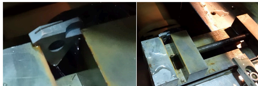
Figure 23. Electro-spark discharge machining of the backing shim.
