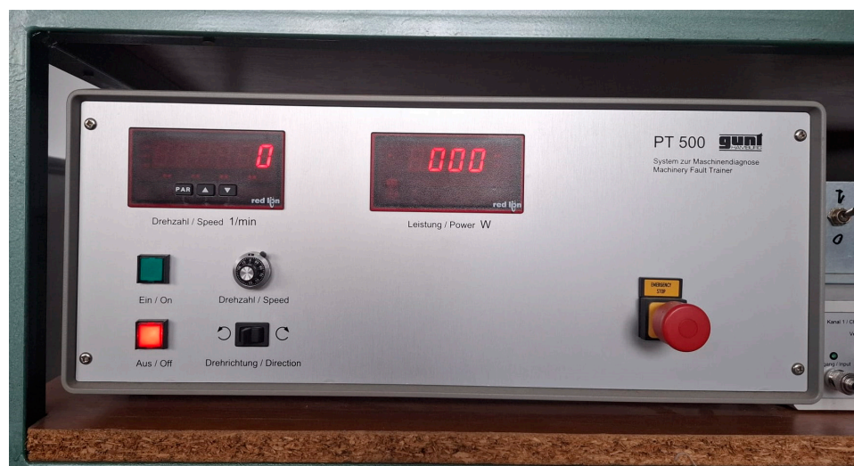
Figure 2. Controller of the electrical motor.
