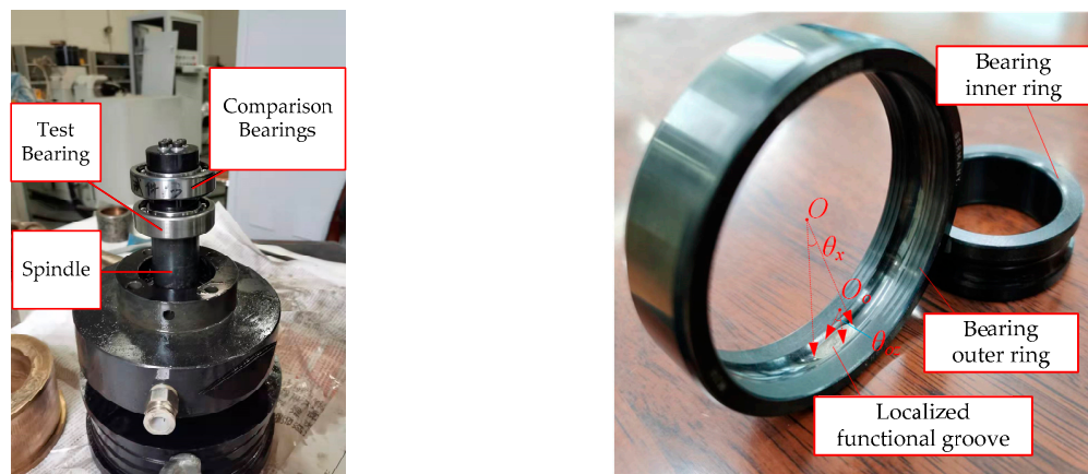
(a) Installation of experimental bearings and comparative bearings (b) Close-up of bearing outer ring
