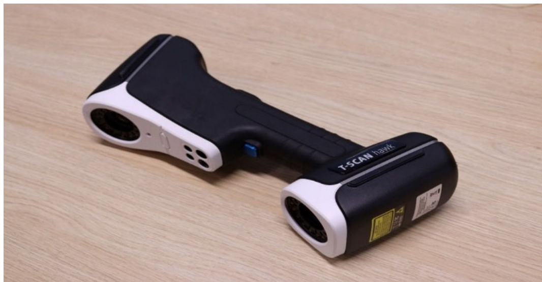
Figure 3. Zeiss T-Scan Hawk 2 handheld laser scanner used for digitizing the damaged component.
