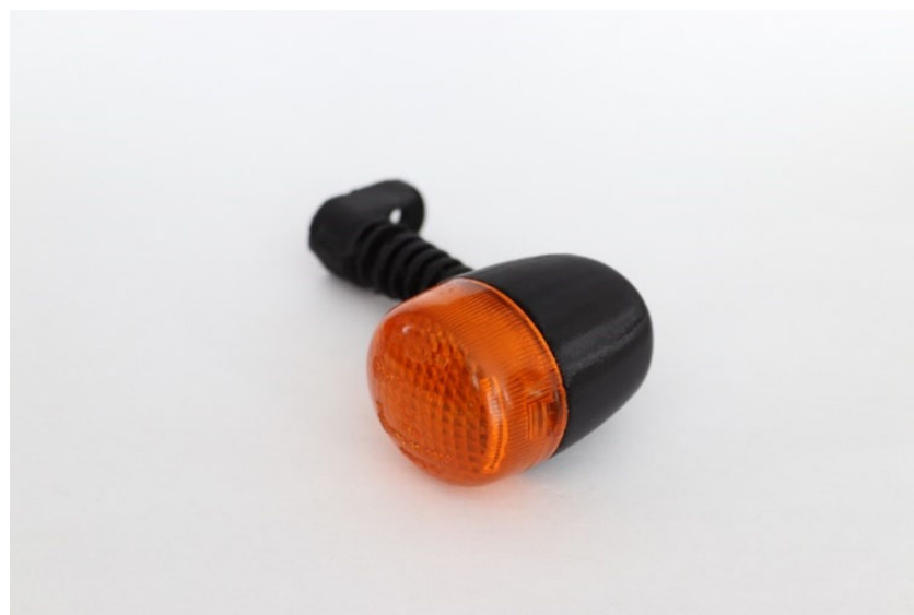
Figure 7. Final 3D-printed component manufactured using continuous fibre-reinforced additive manufacturing.
