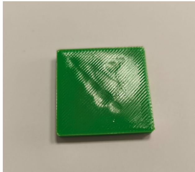
Figure 4. Burnished sample with a force of 25 N.
