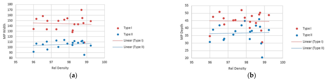
Figure 9. Effect of relative density, \rho_{rel} [%], on melt pool (SSR = 90^\circ ) (a) width [ \mu\text{m} ] and (b) depth [ \mu\text{m} ].
