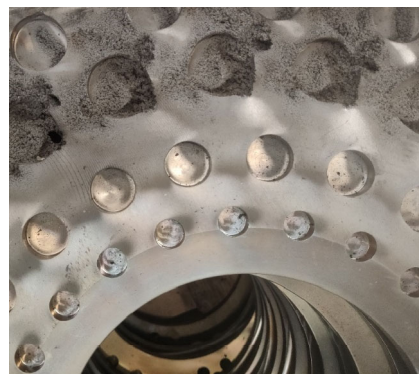
Figure 13. Cavitation corrosion of model hydraulic dynamometer.
