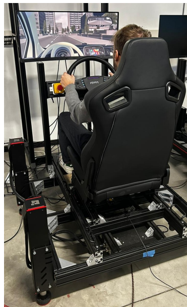
Figure 23. Experimental setup of a driving simulator exploiting the 3-DoF, 4-legged PKM.
