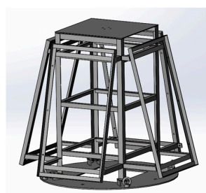
Figure 4. Support frame of the power equipment.
