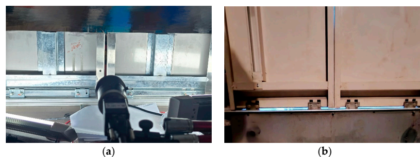
Figure 14. Data acquisition scenes: (a) Simulated landing door inspection platform; (b) In-shaft landing door image with safety keeper.
