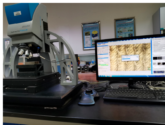
Figure 17. Surface topography measurement of machined surface of fan blisk blade.
