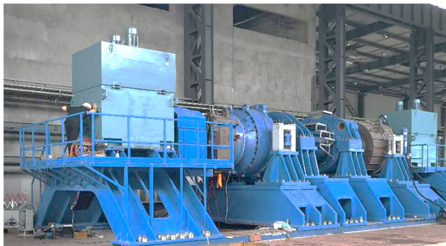
Figure 15. The asymmetrical planetary gear system experimental platform.
