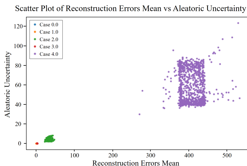
Figure 19. Aleatoric uncertainty vs. mean reconstruction error for different cases of unbalance fault.
