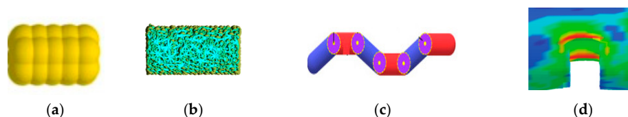
Figure 2. Simulation models of crop straw. (a) Multi-sphere rigid particles (b) Bonded contact model (c) Model of multi-segment rigid sphere-cylinder elements (d) Straw finite-element model. The color in (b) represented the bonding contacting positions; (d) The color represented the distribution of stress.
