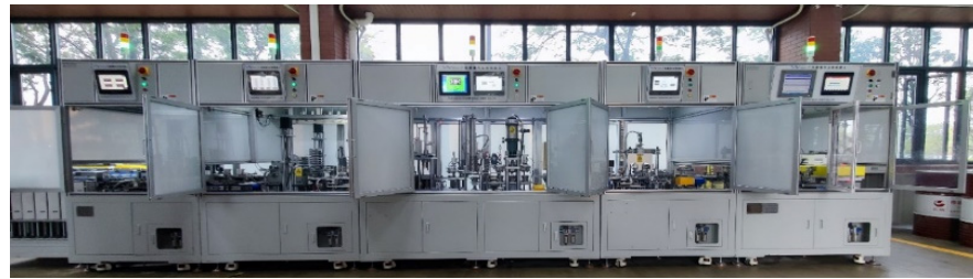
Figure 4. Intelligent assembly line of bearing components.
