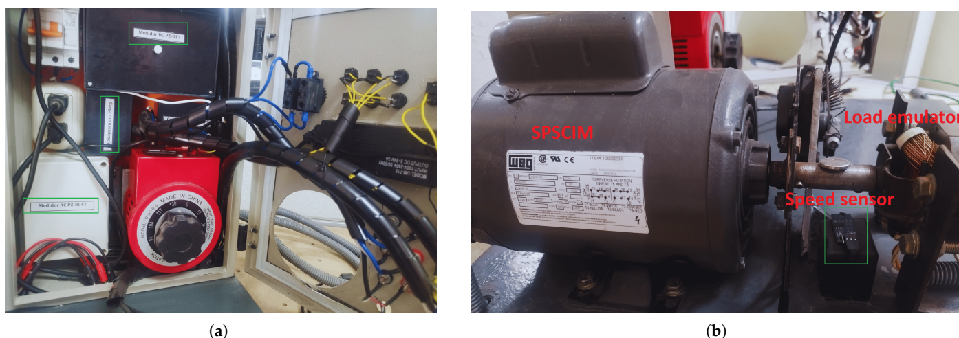
Figure 4. Description of the test station: (a) Internal distribution and connection of the test module. (b) Mechanical coupling between the SPSCIM and the load emulator.
